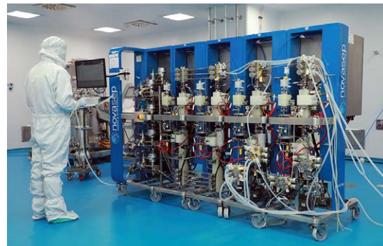
An Enzene technician operates a multicolumn chromatography set-up.
